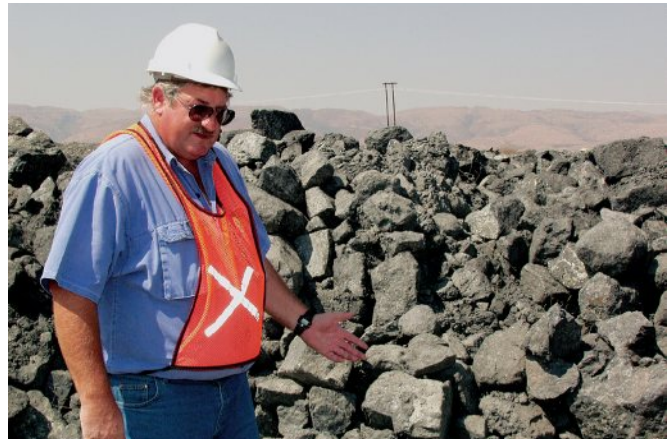
Charles Butler stands next to a chrome ore stockpile. The even breaking qualities of the power deck blasting system give a relatively uniform lump size creating a more marketable product.
